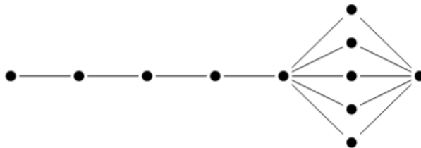
Figure 18: A graph where a BFS will have to search through the same tail on the left for every path.
